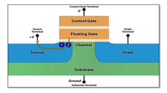
A4578; SVA Ch. 7. The dopants in regions 1 and 2 cause the electrons to move on the desired path (the yellow line) through and out the source. A156 (col. 7, ll. 14-20). In theory, having the two doped regions arranged in this manner reduces leakage out through the substrate. A153 (col. 1, ll. 12-15).
