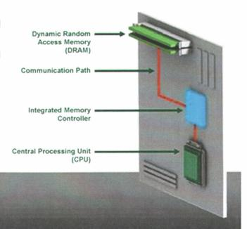
As the picture shows, the DRAM communicates with a memory controller that, in turn, communicates with the CPU. Today, the memory controller is physically part of the same chip as the CPU. A Graphical Processing Unit ("GPU") is a special computer brain for complex graphics, such as those used in video games, and operates in essentially the same way. *See generally* A2889-3207.
