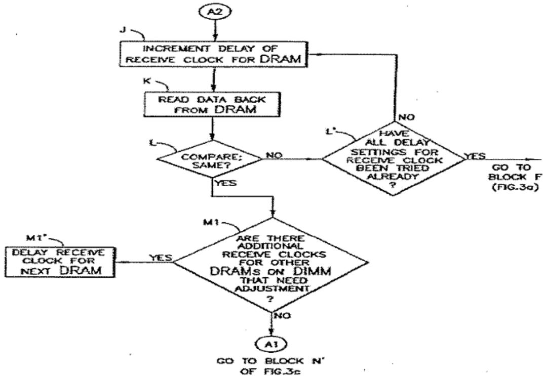
Ad132. See A40642-43 (12:61-14:24). Under this algorithm, the amount of signal delay is changed if the data received from the DRAM at device start-up does not match the test data stored in the controller. See Ad132.
