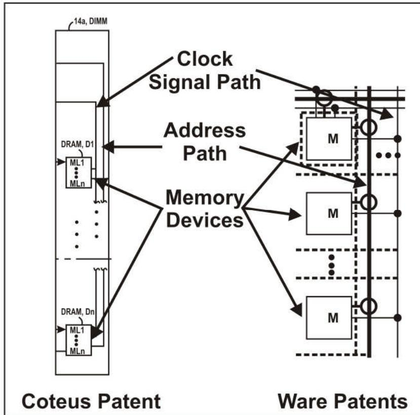
The two drawings describe functionally identical circuits arranged in the same way. Both drawings show multiple memory devices connected serially along clock lines and address lines. If, as Rambus urges (at 41), the Coteus control (clock and address) lines are equalized, then so too are the same lines in the Ware patents. Instead, the ALJ properly judged that the specification and the drawings of both patents disclose lines of varying lengths.
